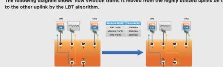
NIOC allows administrator to allocate I/O shares to different traffic types similar to allocating CPU and memory resources to a virtual machine • Following traffic types are supported : Fault Tolerance, iSCSI, vMotion, Management, vSphere
