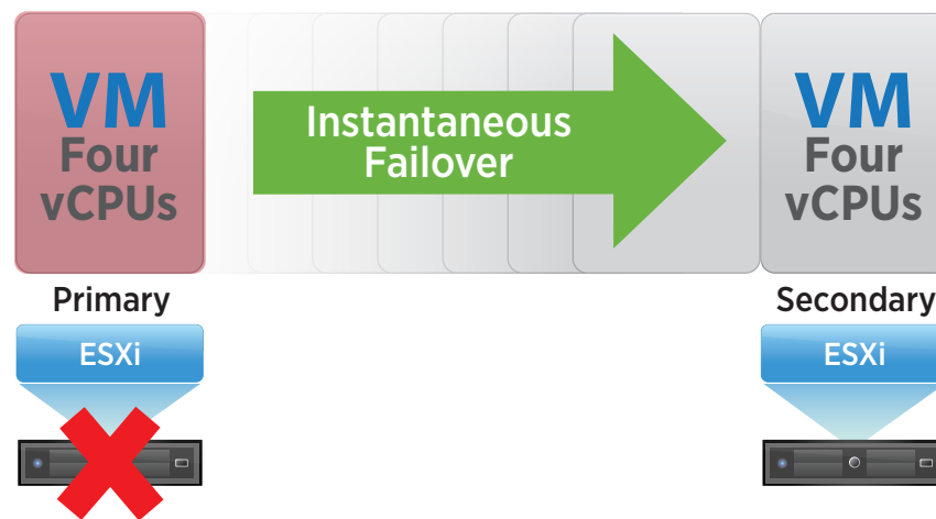
Figure 3. vSphere Fault Tolerance for ASCS Protection
